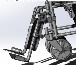
But when we lift the steering tube and leg support so that the boss is no longer stuck in the groove and rotate the steering tube and leg support so that the boss is stuck in the front groove, then we realize our goal to put the leg support under the wheelchair. The detailed SolidWorks file will be uploaded with the individual analysis.
