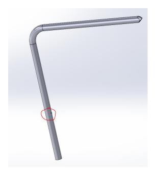
The trick of my design which can rotate the leg supports under the wheelchair is to adjust the position of the boss in the groove. The leg support is in its normal use when the boss is stuck in the back groove of the steering tube.
